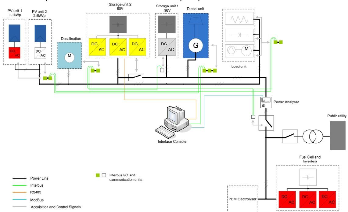
**Fig.1** Block diagram of the Hybrid system and Microgrid test site of CRES
