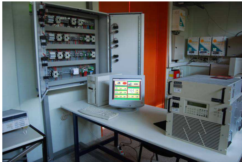
Fig. 1 Programmable Grid simulator and load-bank control
