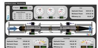
Labview interface for the monitoring of the microturbine
