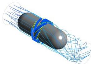
Numerical simulation of flow into a counter-rotating microturbine
