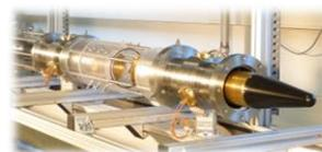
Counter-rotating micro-hydro turbine - Bulb version
