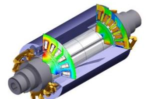
Electrical generator of the counter-rotating microturbine
