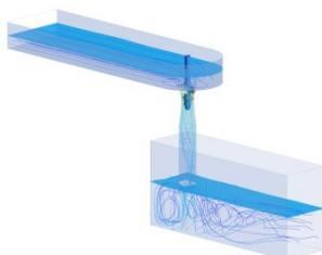
Numerical simulation of flow into a full picoturbine
