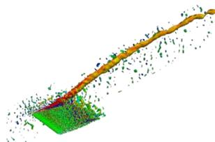
Numerical simulation of a Kaplan turbine tip vortex
