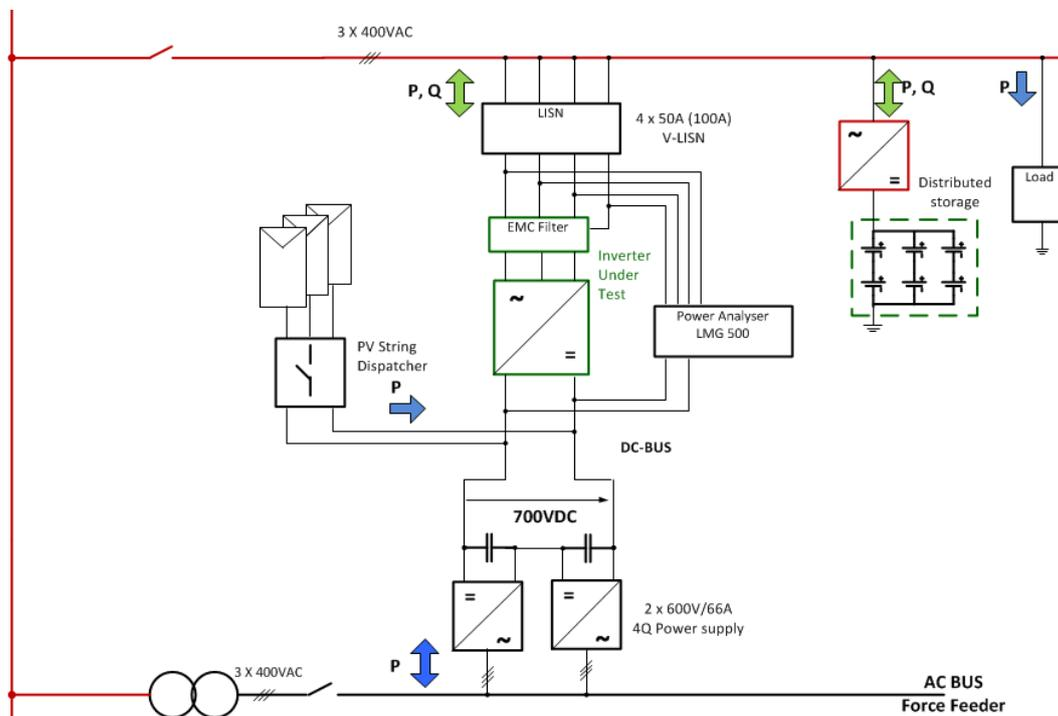
Figure 8: Test bench for individual Active In-feed converter
