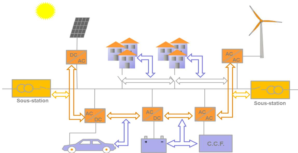
**Figure 2: Electrical distribution and communication systems in GridLab Low Voltage**
