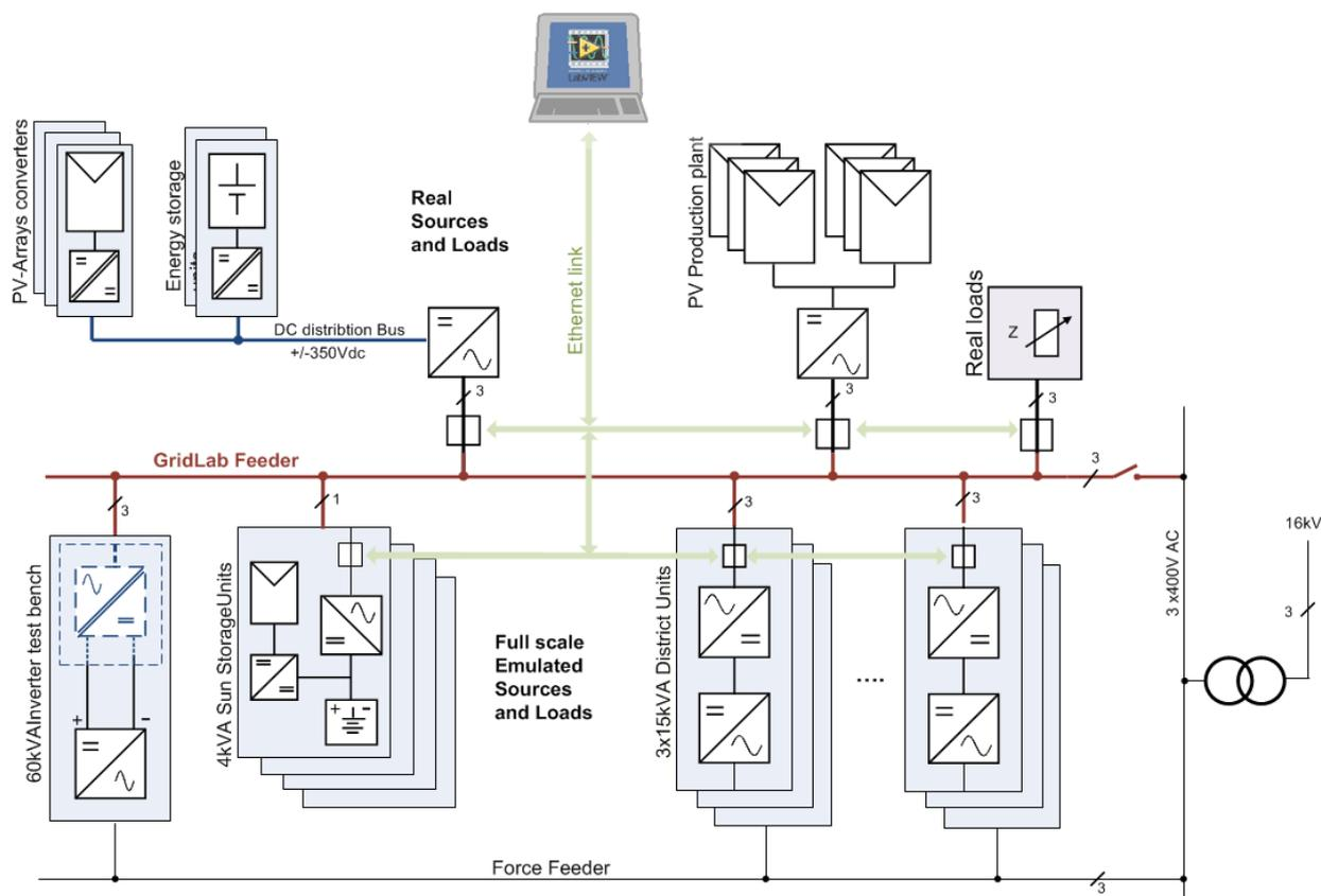
Figure 4: Simplified block diagram of GridLab Low Voltage infrastructure
