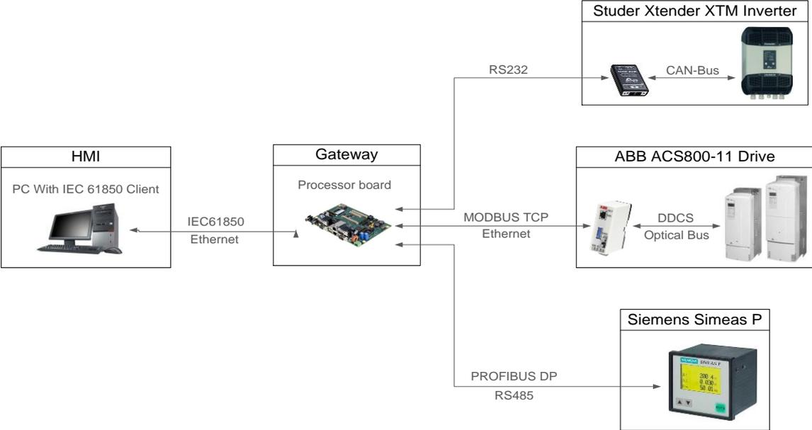
Figure 6: ICT infrastructure for the GridLab Low Voltage
