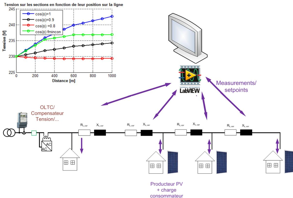
**Figure 3: Control of the 3 x 15kW district Unit for a grid control strategy scenario**
