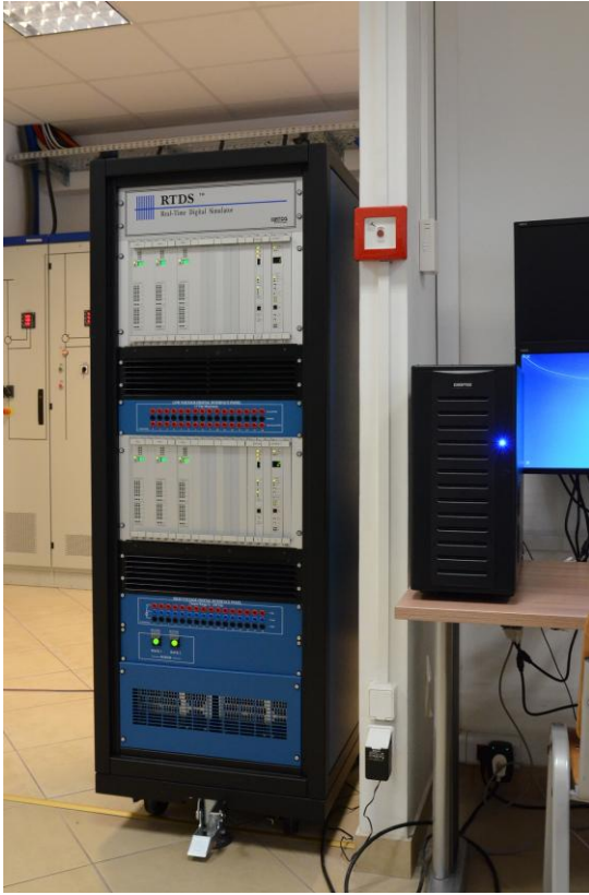
Photograph: Real Time Digital Simulator - RTDS (DER laboratory at TU Lodz)
