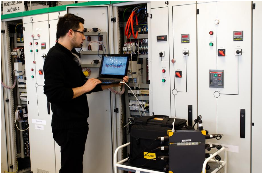
Photograph: Power quality analyzers Fluke 1760 (DER laboratory at TU Lodz)
