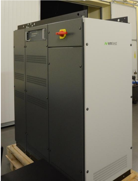
Photograph: Multifunctional 3-phase AC/DC source with power recovery module up to 60kVA (DER laboratory at TU Lodz)
